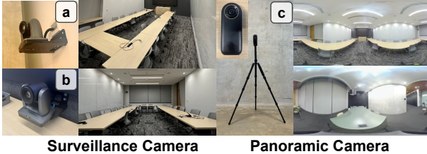
Figure 10: The camera setup for obtaining visual priors.
