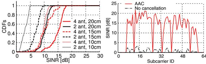
(a) Under different Tx antenna number & interfering distance. (b) Receiving SINR on 64 OFDM subcarriers (20MHz channel).
