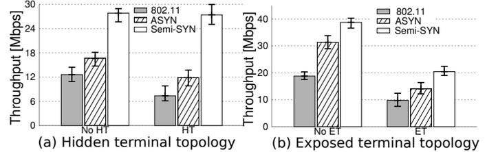
Fig. 8: Throughput comparison between different contention mechanisms, with and without hidden/exposed terminals.
