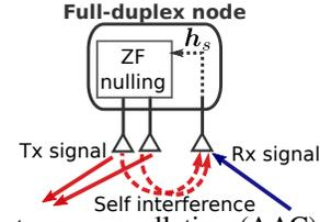
Fig. 5: Active antenna cancellation (AAC) over MU-MIMO.
