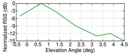
Figure 14: Effect of radar/metasurface height mismatch
