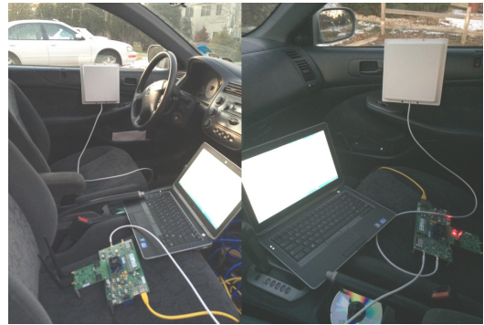
Figure 8. Experimental setup for gesture recognition inside a conventional Car.
