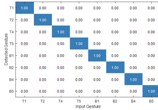
Fig. 19. Confusion matrix for detecting eight selected keys.
