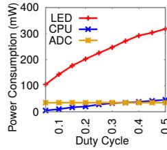
Figure 25: A breakdown of Okuli's power consumption.
