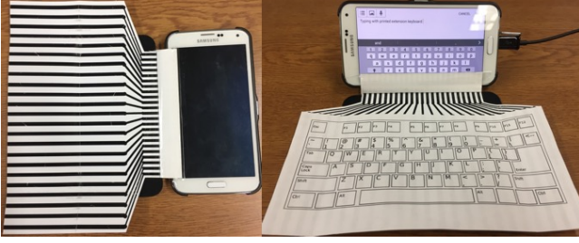
Figure 28: Customized printed extension to extend the interaction area of smart phone. The extension is integrated with a flip cover phone case, and can be folded to fit inside the cover. Keyboard layout printed on normal paper attached on top of conductive stripes.
